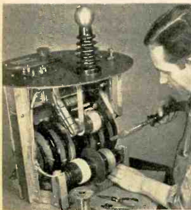
Real high power! Putting the finishing touches on a transformer which is to deliver 60,000 volts at 0.05 amps
