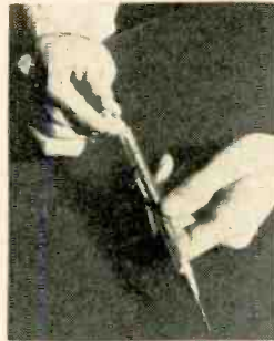
A "solder pencil", developed by GE keeps the solder free from dirt and handling by the worker
